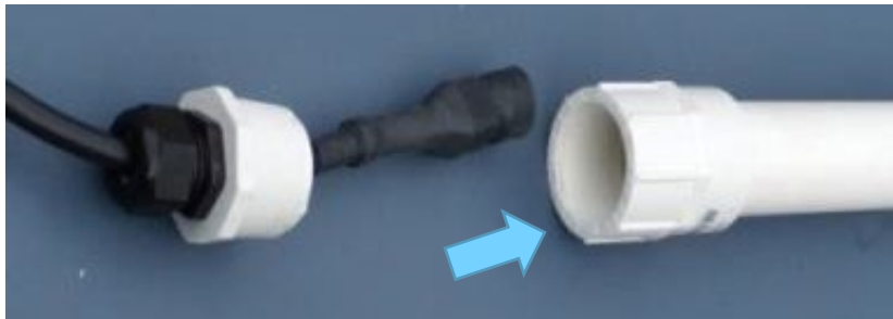
Top End of PVC Handle with newly bonded adapter
