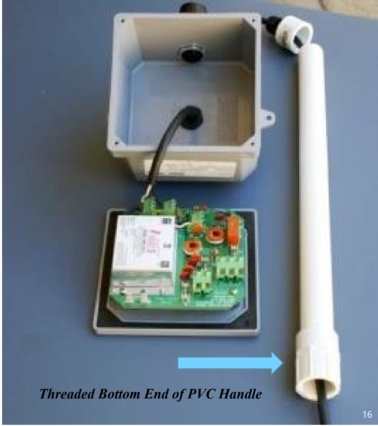
Top End of PVC Handle with newly bonded adapter
